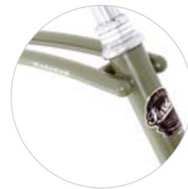
The Parabike features a unique duplex-tube frame, giving a comfortable ride and unmistakable style. The design harks back to the paratroop Airborne cycles used by the British Army in World War II.
