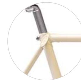
Both Clubman frames feature classic geometry made from Reynolds 531 tubing with investment-cast cut-away lugs and cast dropouts with mudguard eyes. The fork has Reynolds taper gauge oval blades with investment-cast crown and a small classic radius bend.
