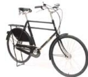
The Roadster also comes in a double-top-tube version for the taller gent. With a frame size of 24.5 inches this superbly crafted machine will suit an inside leg of 35 inches upwards and give the rider the stability and control a double-top-tube can provide.
