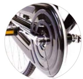
A fully enclosed chaincase protects you and your bike from unwanted grease and grime. This helps to reduce wear and tear on the chain and decreases the amount of maintenance that your bike will require.
