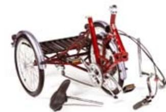
The Tri-1 has the option of a hinged frame that allows the trike to be folded quickly for easy storage or transportation. The folded trike will fit into most cars. A propstand is provided to keep the trike upright when folded.
